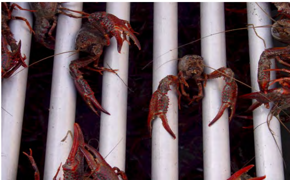
Figure 3. Size grading in crawfish is accomplished according to width of the carapace.
